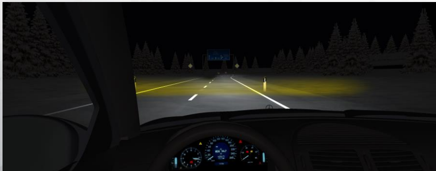
Rigid D-series SAE Fog Coverage is small. Narrow and skinny. Moderate mid-distance selective illuminance
