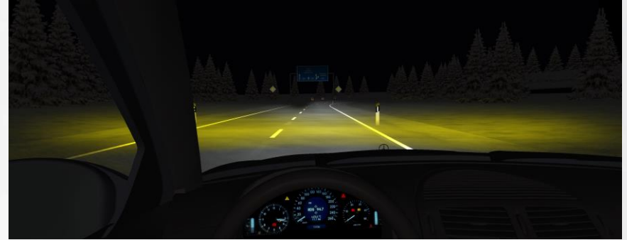
SS3 Max ABL SAE Fog Strongest far road-edge illuminance, lack of foreground and mid-distance filling capability, peaky band shaped illuminance.
