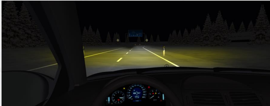
4 Banger NCS Wide Scaled down illuminance impression of HXB Wide. Blends with low beam at neutral illuminance balance.
